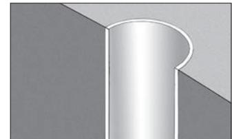
After concrete is complete, use an EZ Stroke pipe saw to cut flush with concrete. The inside pipe fit drain/cleanout can easily be glued into the pipe.
