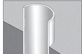
The concrete should be poured so that the pipe stack is above the finished surface.
