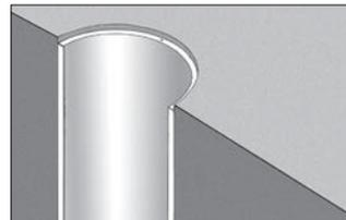
After concrete is complete, use an EZ Stroke pipe saw to cut flush with concrete. Then, use a socket saver or inside pipe cutter to trim pipe 3/8" below concrete surface.
