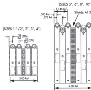
DESCRIPTION: Couplings consist of gasket and shield assemblies, the shield assemblies have four or six clamps depending on size. The clamps are fastened with eyelets to the bi-directional corrugated shield.
