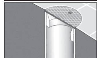
Lay tile to the edge of the cover or strainer. No chisel or tape needed!
