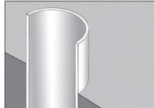
The concrete should be poured so that the pipe stack is above the finished surface.
